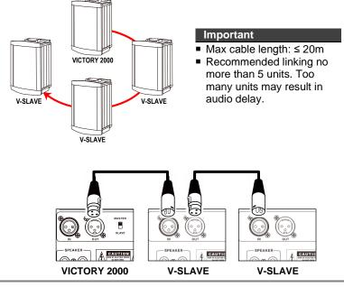
2 Turn on master POWER of VICTORY 2000 and then adjust SLAVE volume control to desired level. The power of V-SLAVE(s) will be automatically activated as soon as the VICTORY 2000 is turned ON, regardless of whether the V-SLAVE's power switch is OFF or ON. The V-SLAVE's volume can be individually adjusted on its control panel.
