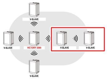
For this purpose, please install a repeater module on the SUB-MASTER unit and a receiver module on SUB-COMPANION units (same procedures as STEP 1 & 2). Both repeater and receiver module must be the same channel and same frequency which must be different from former repeater and receiver module.
