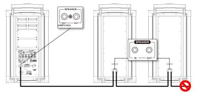
2 There are two output jacks for external speakers. When connected from the LEFT one (SWITCHED), the V-SLAVE will be MUTED and only the external speaker V-SP will broadcast. When connected from the right jack, both the V-SLAVE and V-SP will broadcast.
